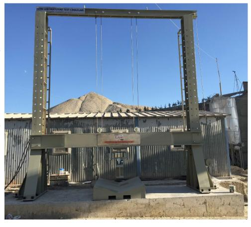
The frames are rigid 2 column constructions with superior axial and lateral stiffness and are precision aligned.
