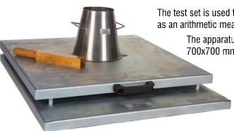
The test set is used for concrete mixes of high workability. The test determines flow index as an arithmetic mean of the diameter of the specimen after working on a flow table.
