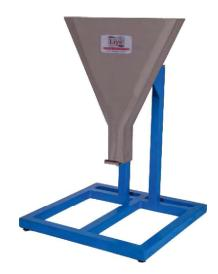
The apparatus is used to evaluate the segregation resistance of freshly mixed self-compacting concrete by the observation the flowing speed due to the difference of samples remaining period in the funnel.
