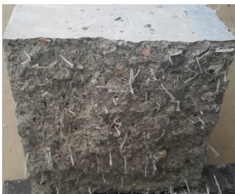
LEKSO 410 presents homogeneous and random fibre dispersion with an appropriate mix design (4 kg/m 3 fibre dosage)
