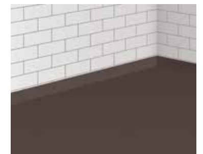
10 Finished waterproofing membrane ready to receive finishes
