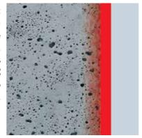
Inside the capillary pores the chemicals react with the free lime and moisture forming insoluble crystals. The mechanism moves further into the concrete, sealing the pores.
