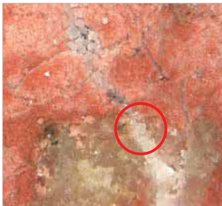
Crack healing by auto-reactive function in the concrete
