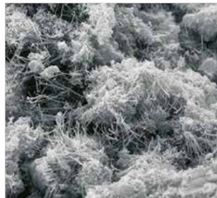
Pore blocking crystals (approx. 5000 times magnification)
